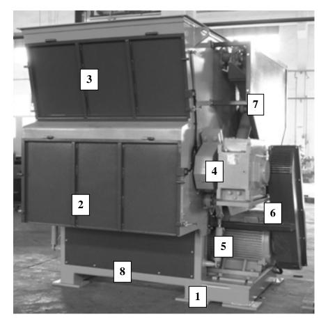
The machine housing, drive motor, gear box, hydraulic system and terminal box are mounted on the base frame for electrical connections.
